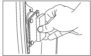
To open the driver side rear door, pull the latch release at the inside edge of the door.
